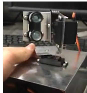
FIGURE 1. CONFIGURATION I ILLUSTRATING THE LIDAR-LITE V3 RANGEFINDER AND THE TWO TOWERPRO SERVOS ON A BENT ALUMINUM BASE.
